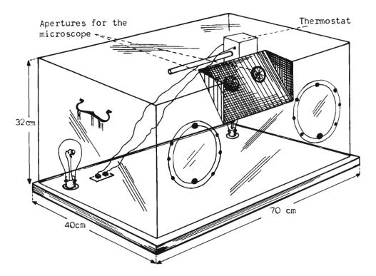
Such a chamber allows a constant temperature to be kept in a very small volume and avoids one remaining for a long time in the confinate isotherm rooms.
